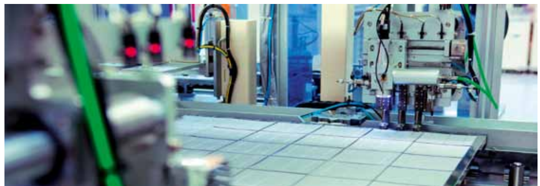
Soldering cell strings
